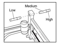
differ depending on which ends of the incline legs are inserted. Set the cross-country skier upright. For a low incline level, insert the incline legs into the top of the front stabilizer, with the front stabilizer resting on the floor.
